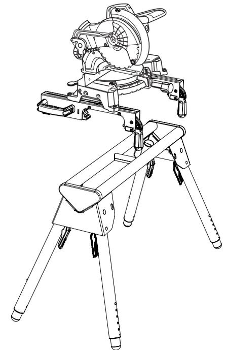
**NOTE:** The saw should be removed from the tool mounts before attempting to tighten or loosen the tool mount adjustment screws.
